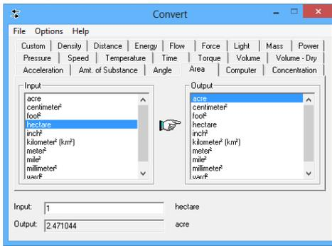
**Convert** is a tool to assist with unit conversion calculations.
