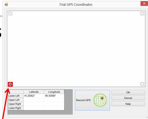
Touch Tablet GPS button to read current position for indicated corner (e.g. LL)
